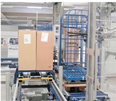
Completely automated storage, order picking, and consolidation of quarter and half pallets
